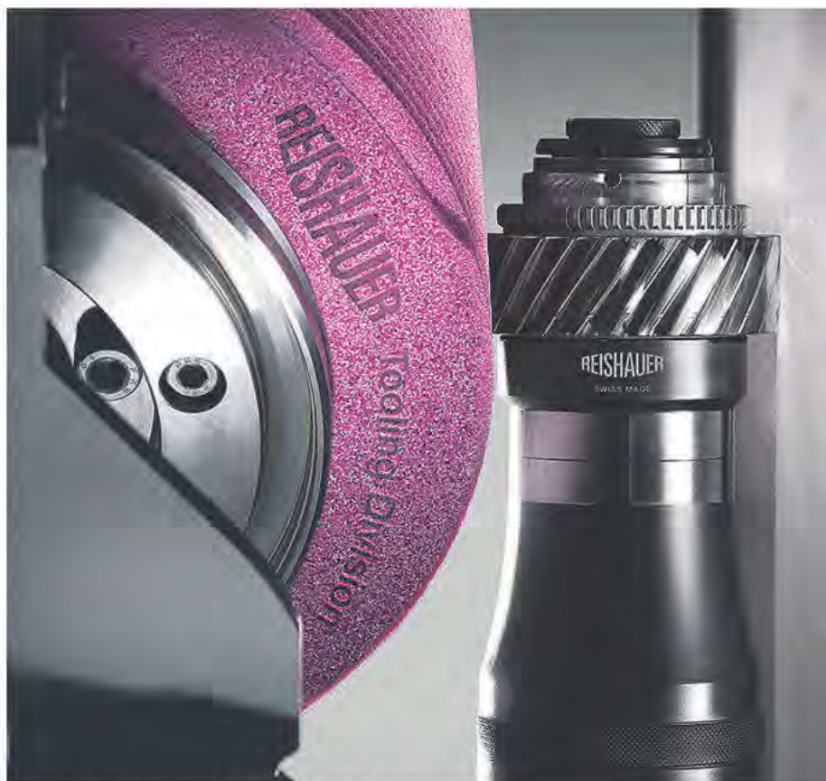
Illustration 1: Continuous generating gear grinding process
