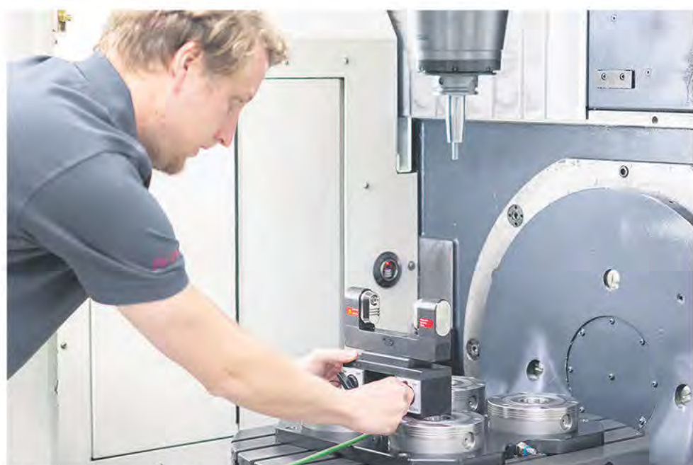
Part of the system is the LC50-DIGILOG laser measurement system known from machining centres. It can be easily attached to the machine processing table by means of a magnetic holder.
