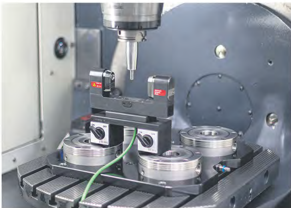
Portable SpindleControl allows non-contact measurements of run-out, vibration, thermal stability and spindle parameters throughout the entire speed range.
