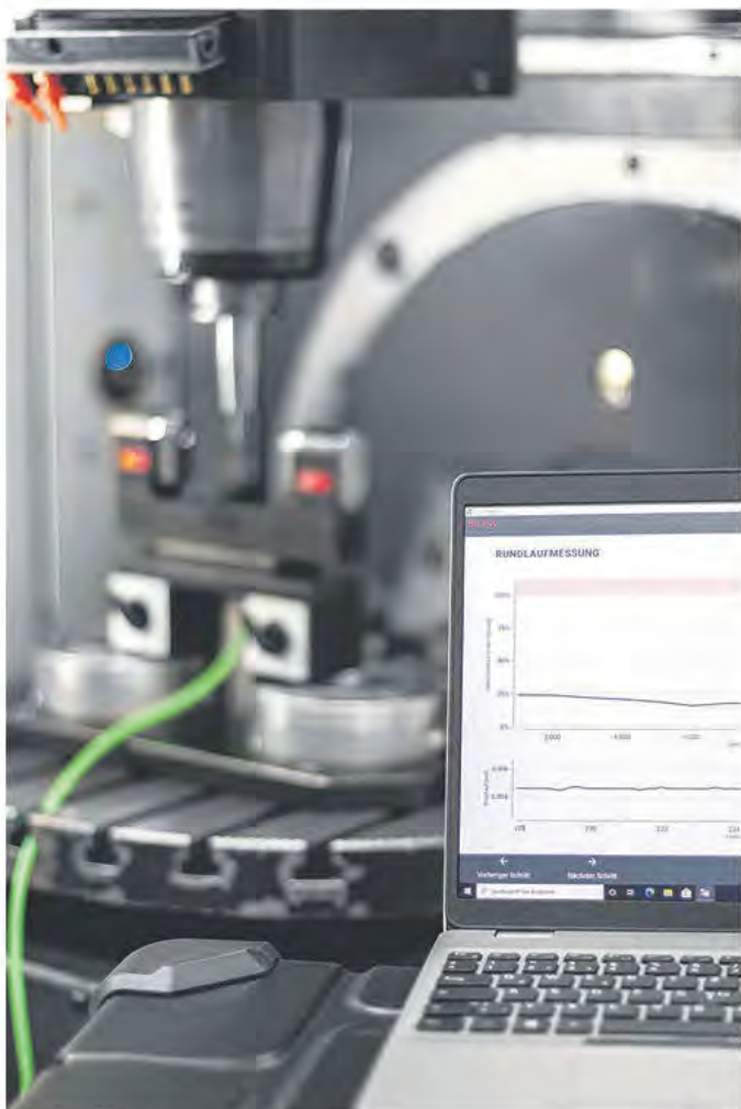
kptec uses Portable SpindleControl (PSC) from BLUM for mobile spindle monitoring. This is a high-precision, portable system for flexible testing and monitoring of motor spindles in machine tools.
