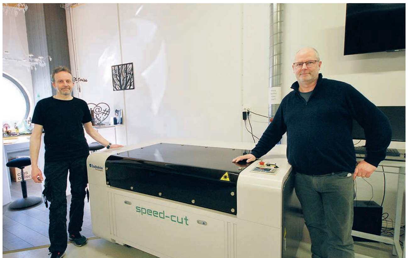
Speed-cut Fiberlaser, SF1313G IPG 1.5Kw. Arbetsyta: 1300mm x 1300mm. Max hastighet: 80m/min. • Max acceleration: 0.8G • 3x400V 16A
