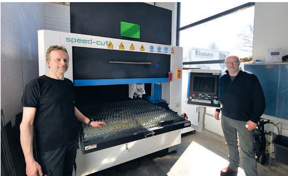
Speed-cut Fiberlaser, SF1313G IPG 1.5Kw. Arbetsyta: 1300mm x 1300mm. Max hastighet: 80m/min. • Max acceleration: 0.8G • 3x400V 16A
